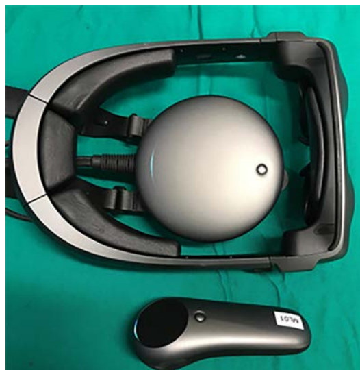
Figure 4 - The Magic Leap 1 is an Augmented Reality device made up of three main components. The Lightwear is the headset that projects 3D digital images into the real world, along with sensors and eye-tracking for environment and user interaction. The Lightpack is a small, wearable processing unit that handles all computing tasks, battery, and runs the device's operating system. The Control is a handheld controller with a touchpad, buttons, motion sensors, and haptic feedback, allowing precise interaction with virtual elements.
