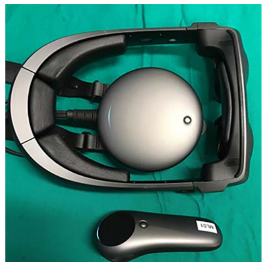
Figure 4 - The Magic Leap 1 is an Augmented Reality device made up of three main components. The Lightwear is the headset that projects 3D digital images into the real world, along with sensors and eye-tracking for environment and user interaction. The Lightpack is a small, wearable processing unit that handles all computing tasks, battery, and runs the device's operating system. The Control is a handheld controller with a touchpad, buttons, motion sensors, and haptic feedback, allowing precise interaction with virtual elements.
