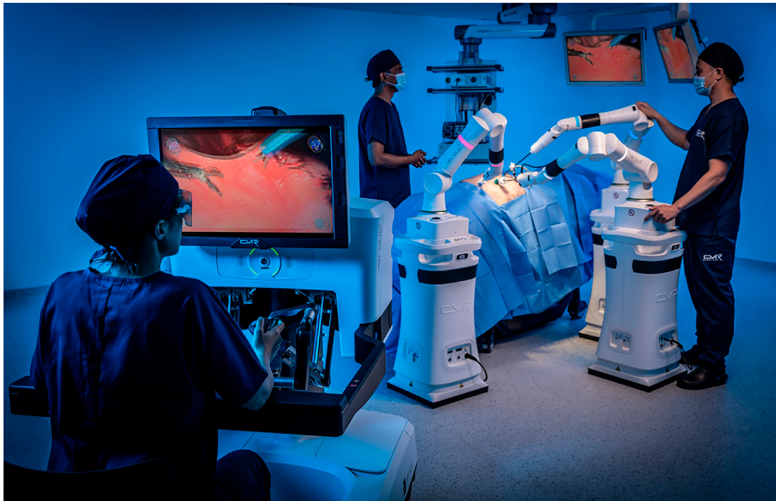
Figure 1 - Console and bedside units.
