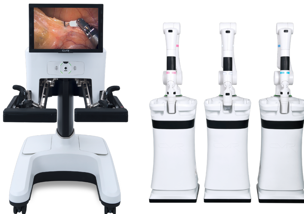
Figure 2 - Open Console with no pedals and docking of modular arms (BSUs).
